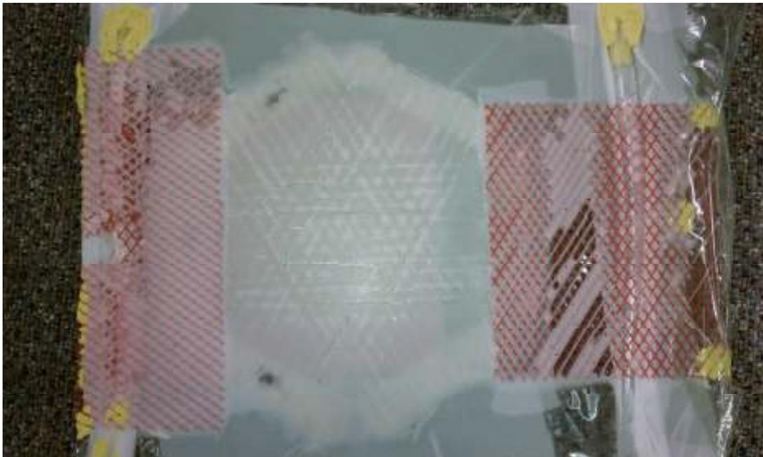
Figure 8: Specimen After Curing with Poor Impregnation
