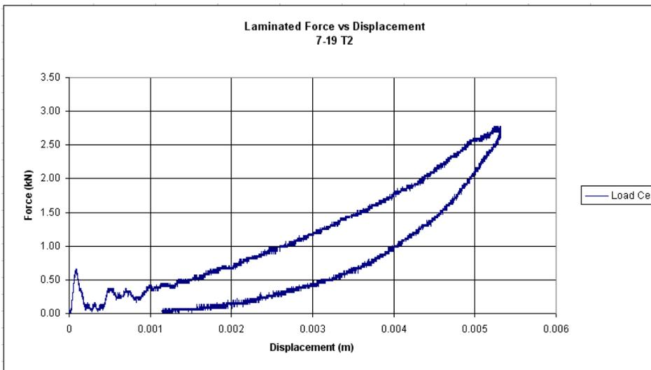
Figure 13-15: Force-Displacement Curves for Laminated Specimens
