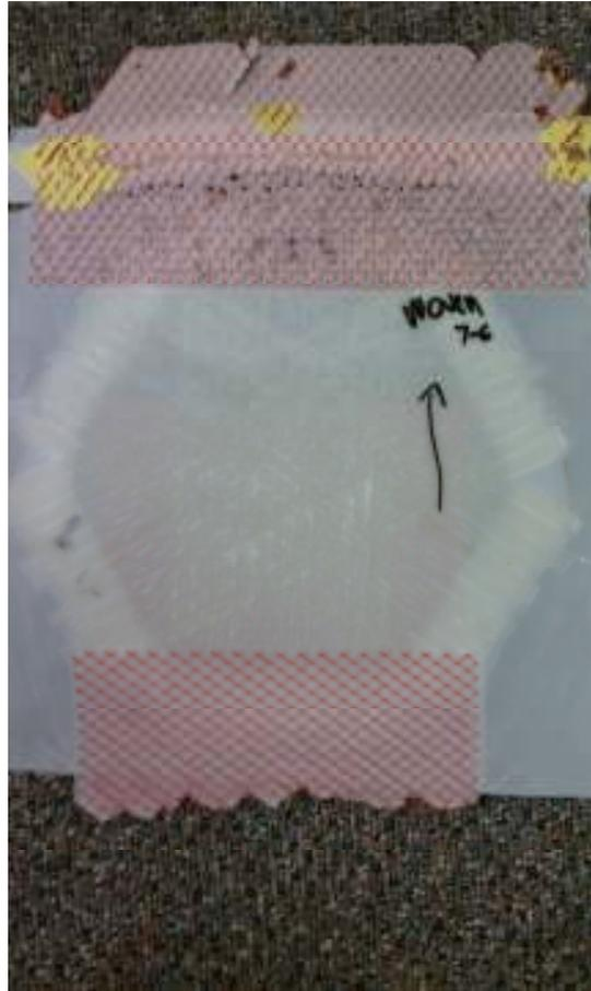
Figure 10: Specimen After Curing with Poor Surface Finish due to Bubbles
