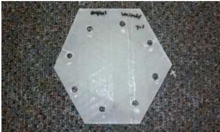
**Figure 12: Specimen Cut and Drilled for Impact Testing**
